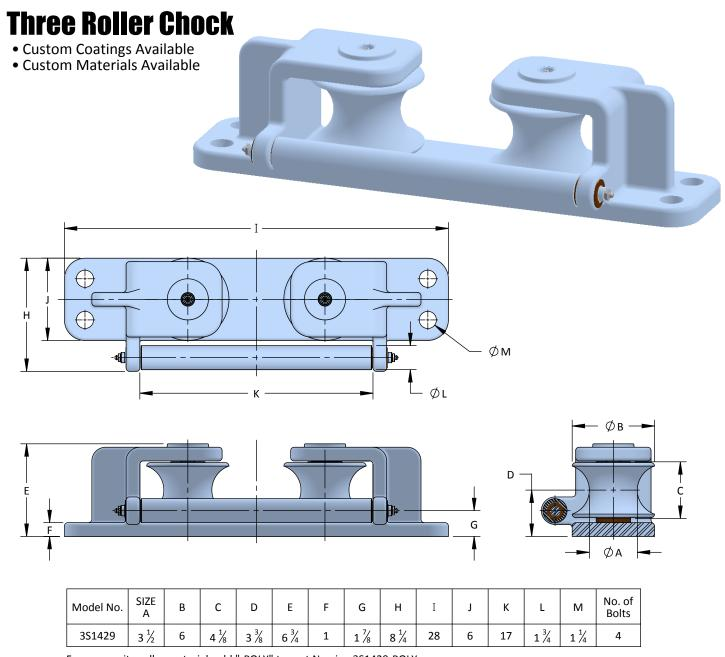
For composite roller material, add "-POLY" to part No., i.e. 3S1429-POLY
